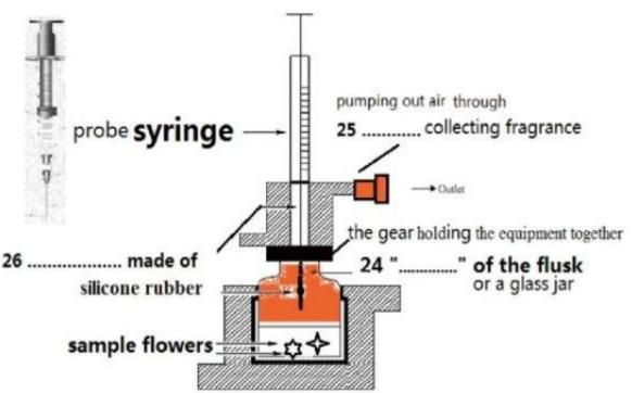
A simple device used to trap molecules
